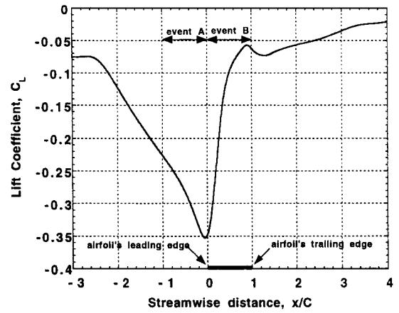
Fig. 10 Time history of the predicted sectional lift for the uncontrolled NACA-0012 airfoil during interaction with an infinite line vortex ( $M_{\infty} = 0.6$ ,  $\alpha = 0$  deg,  $Re = 3 \times 10^6$ ,  $GAM = 0.30$ , and  $rv/C = 0.20$ ).
