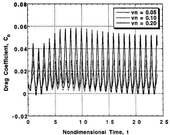
**Fig. 4** Predicted time histories of the sectional drag for the NACA-0012 airfoil—effect of peak jet velocity ( $M_{\infty} = 0.6$ ,  $\alpha = 0$  deg,  $Re = 3 \times 10^6$ , and  $f = 1585$  Hz).
