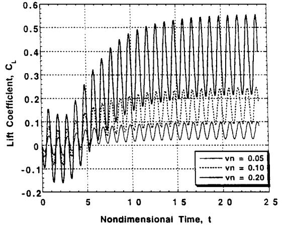
**Fig. 3** Predicted time histories of the sectional lift for the NACA-0012 airfoil—effect of peak jet velocity ( $M_{\infty} = 0.6$ ,  $\alpha = 0$  deg,  $Re = 3 \times 10^6$ , and  $f = 1585$  Hz).
