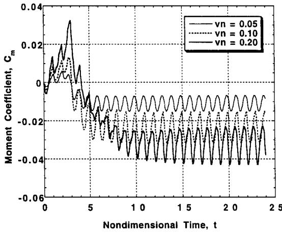
Fig. 5 Predicted time histories of the pitching moment for the NACA-0012 airfoil—effect of peak jet velocity ( $M_{\text{inf}} = 0.6$ ,  $\alpha = 0$  deg,  $Re = 3 \times 10^6$ , and  $f = 1585$  Hz).
