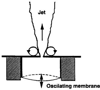
Fig. 1 Sketch of a zero-net-mass synthetic jet actuator
