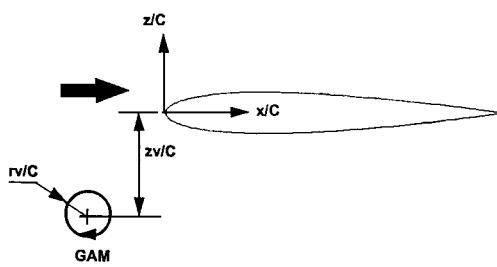
Fig. 9 Sketch of the model airfoil-vortex interaction problem.
