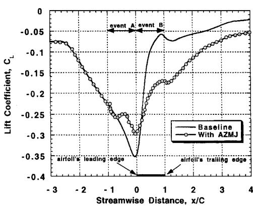
Fig. 12 Predicted sectional lift coefficients for the uncontrolled and controlled airfoil-vortex interaction problems ( $M_{\infty} = 0.60$ ,  $\alpha = 0$  deg,  $Re = 3 \times 10^6$ ,  $GAM = 0.30$ ,  $rv/C = 0.20$ ,  $vn = 0.20$ , and  $f = 1585$  Hz).
