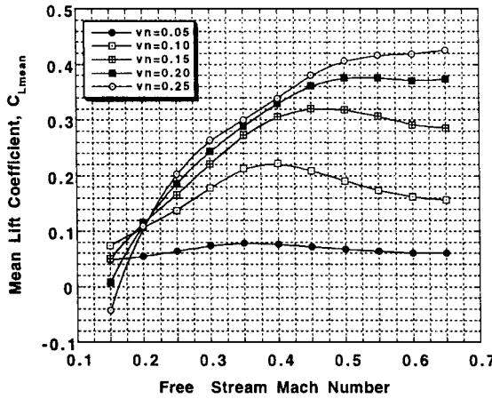
Fig. 6 Predicted mean sectional lift values for the NACA-0012 airfoil—effect of freestream Mach number ( $\alpha = 0$  deg,  $Re = 3 \times 10^6$ , and  $f = 1585$  Hz).
