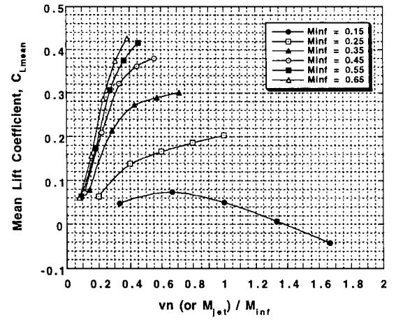
Fig. 7 Predicted mean sectional lift values for the NACA-0012 airfoil—effect of Mach-number ratio ( $\alpha = 0$  deg,  $Re = 3 \times 10^6$ , and  $f = 1585$  Hz).
