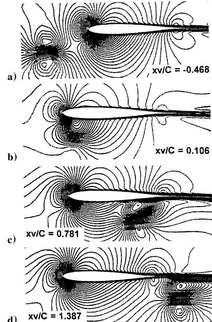
Fig. 11 Predicted Mach-number contours for the uncontrolled NACA-0012 airfoil during interaction with an infinite line vortex ( $M_{\infty} = 0.6$ ,  $\alpha = 0$  deg,  $Re = 3 \times 10^6$ ,  $GAM = 0.30$ , and  $rv/C = 0.20$ ).
